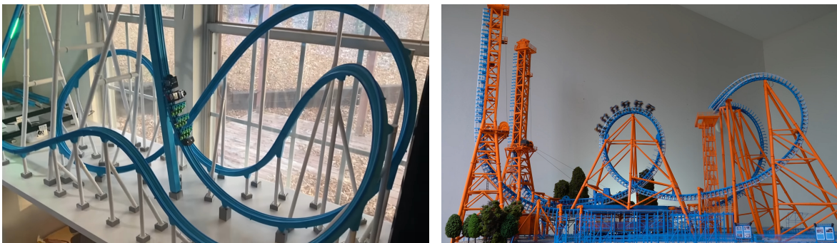
Figure 2: Two 3D-printed models, motorized and driven electronically. (Left) An original layout, motion-controlled with a rack-and-pinion [3]. (Right) A 1:45-scale recreation of Stunt Fall, controlled with a loop of cable [4]. Images used with permission.
