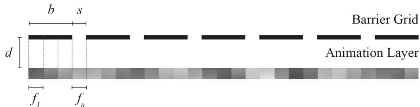
Figure 2: The base schematic setup of Barrier Grid Animation with its main parameters.
