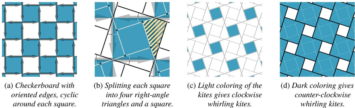
**Figure 2:** Construction of the whirling kites pattern from a square tiling.
