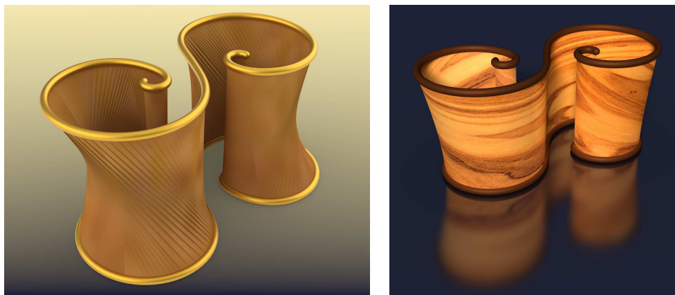
Figure 4: A double-spiral ruled surface, rendered in Rhino (left). Rendered in Photoshop (right).
