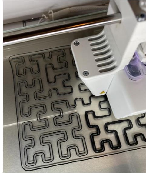
Figure 6: One of the sixteen subsquares printing on an Ultimaker 3
