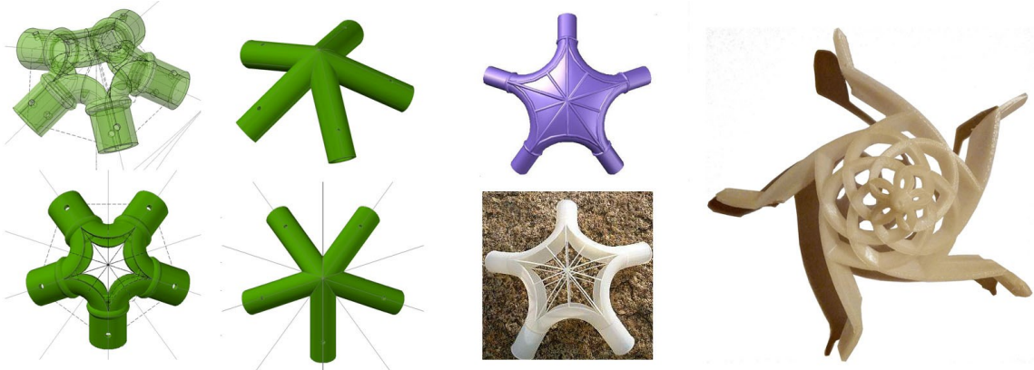
Figure 5: PolyConnec: design digital models and built prototypes
