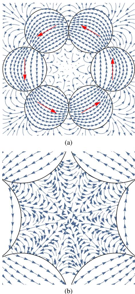
**Figure 10:** Magnetic field from a hexagonal loop on the plane of the loop. Inside each magnet, only the total of the contributions to the magnetic field from all other magnets is shown. Outside of the circles, the total contribution from all magnets is shown. Figure 10b shows a closeup view of the center of the loop.
