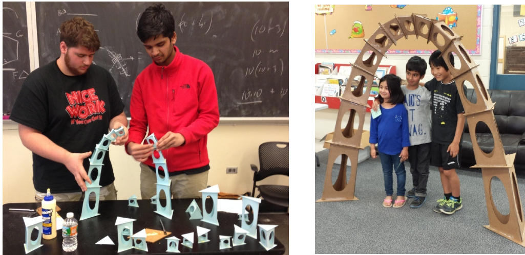
Figure 2: Catenary arches of paper (16 inches tall) and of cardboard (4 foot tall).
