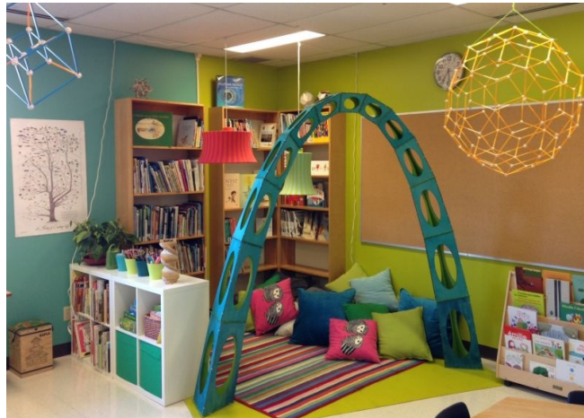
Figure 1: Catenary arch made of laser-cut wood pieces joined with cable ties. (6.5 feet tall)
