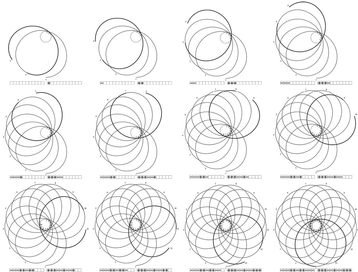
**Figure 2:** Algorithm of assembling and weaving of the cyclic knot with 13 bights and 12 leads.
