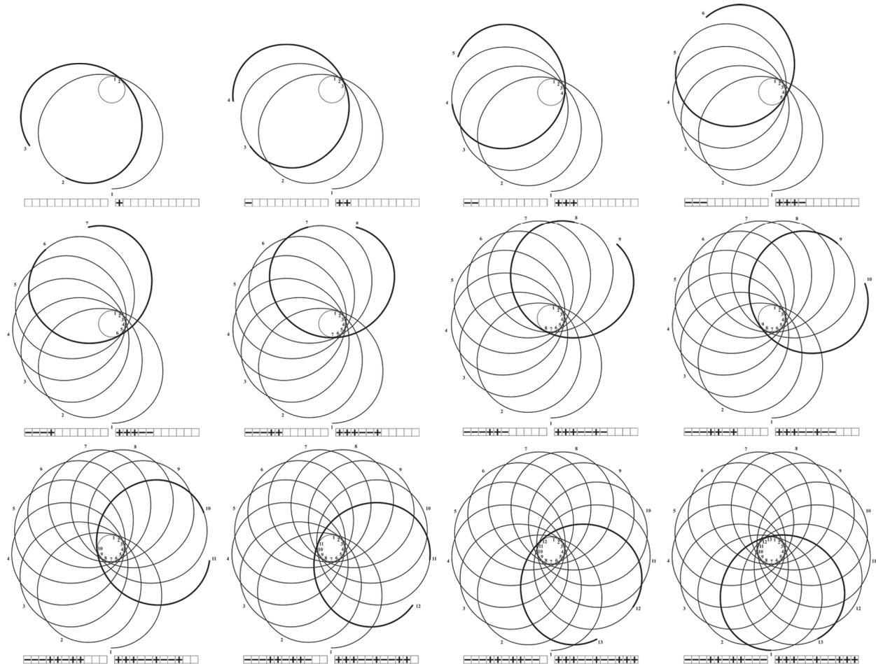
**Figure 2:** Algorithm of assembling and weaving of the cyclic knot with 13 bights and 12 leads.
