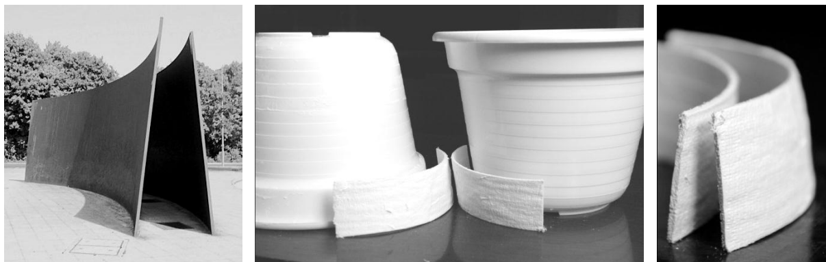
Figure 10: “Berlin Junction” and its simulation with plaster bandages molded over two conical pots.
