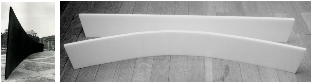
Figure 9: “Tilted Arc” (left) and an easy experiment of stability for straight and curved surfaces. A straight sheet of foam board will easily fall under a gentle blow. The curved sheet will resist the blow or will slide instead of falling.
